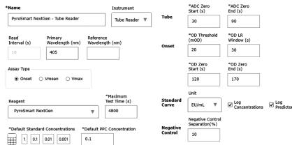
Figure 3: Pyros® eXpress Software Settings for PyroSmart NextGen® Assays
