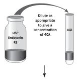
2. From this concentration (e.g.  $40\lambda$ ) prepare a concentration of double the labeled lysate sensitivity ( $2\lambda$ ) in a dilution tube for positive controls. For example:
